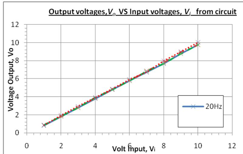
Figure 5 Output voltage outputs ( $V_o$ ) vs. input voltage ( $V_i$ ) for different frequency using circuit
