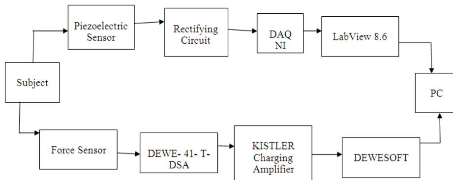
Figure 6: Schematic diagram for the overall experiment
