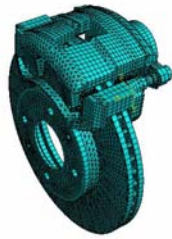
Figure 2: Finite element model of a disc brake assembly
