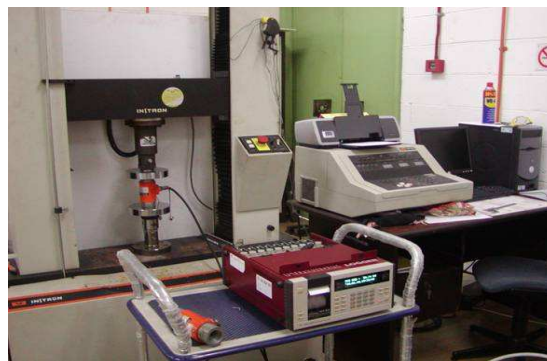
Figure 7: Calibration of 50 kN load cell using 100 kN Instron Universal Testing Machine.
