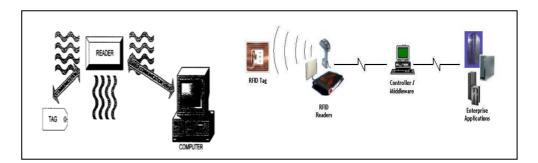
Figure 3: A Typical RFID System [3]
