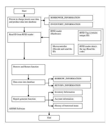
Figure 9: Flow diagram for hardware and software integration
