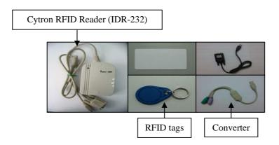
Figure 10: Hardware for ASSMS system
