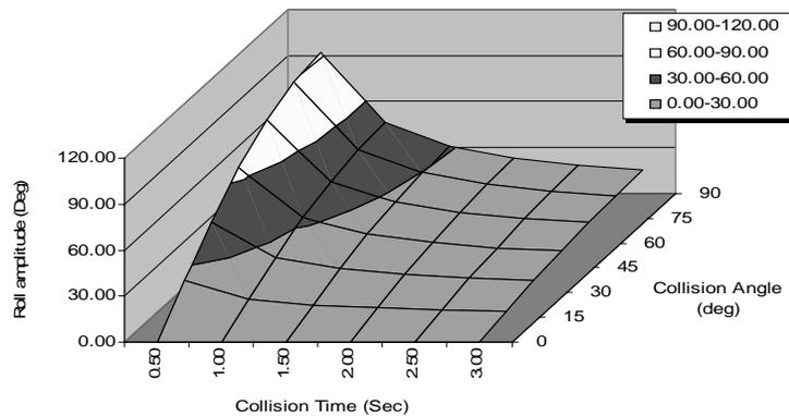
Figure 5: Maximum roll amplitude against collision time and collision angle
