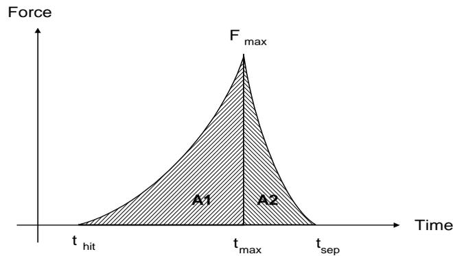
Figure 2: Collision force is an exponential function over the contact period
