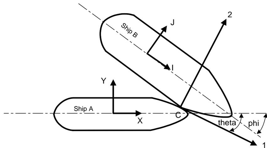
Figure 1: Co-ordinate system of a ship-ship collision
