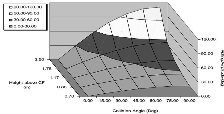
Figure 7: Maximum roll amplitude against collision angle and height of contact point
