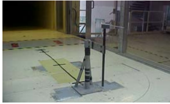
Figure 7: Hotwire during velocity calibration process
