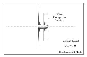
Figure 3: Critical wash pattern for displacement vessels [4]
