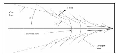
Figure 1: Ship-generated waves [2]
