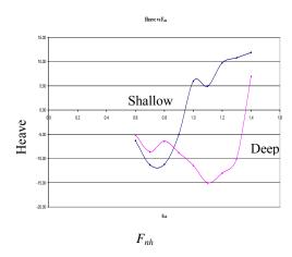
Figure 9: Experimental maximum heave against depth froude number
