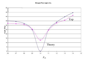
Figure 11: Angle of divergent against depth froude number
