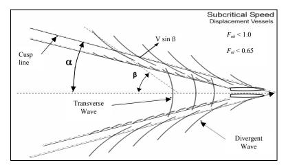
Figure 2: Sub-critical wash pattern for displacement vessels [4]
