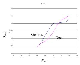
Figure 8: Total model resistance against depth froude number
