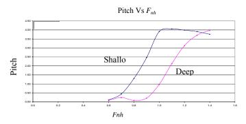
Figure 10: Experimental maximum pitch against depth froude number
