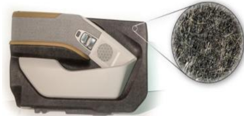
Figure 1: Natural fiber (kenaf) based bio-composite in BMW i3 door panel
