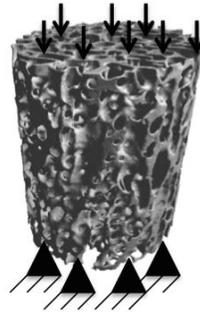
Figure 5: Load and boundary on trabecular bone
