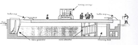
Fig. 1 Cross Section View of the Towing Tank
