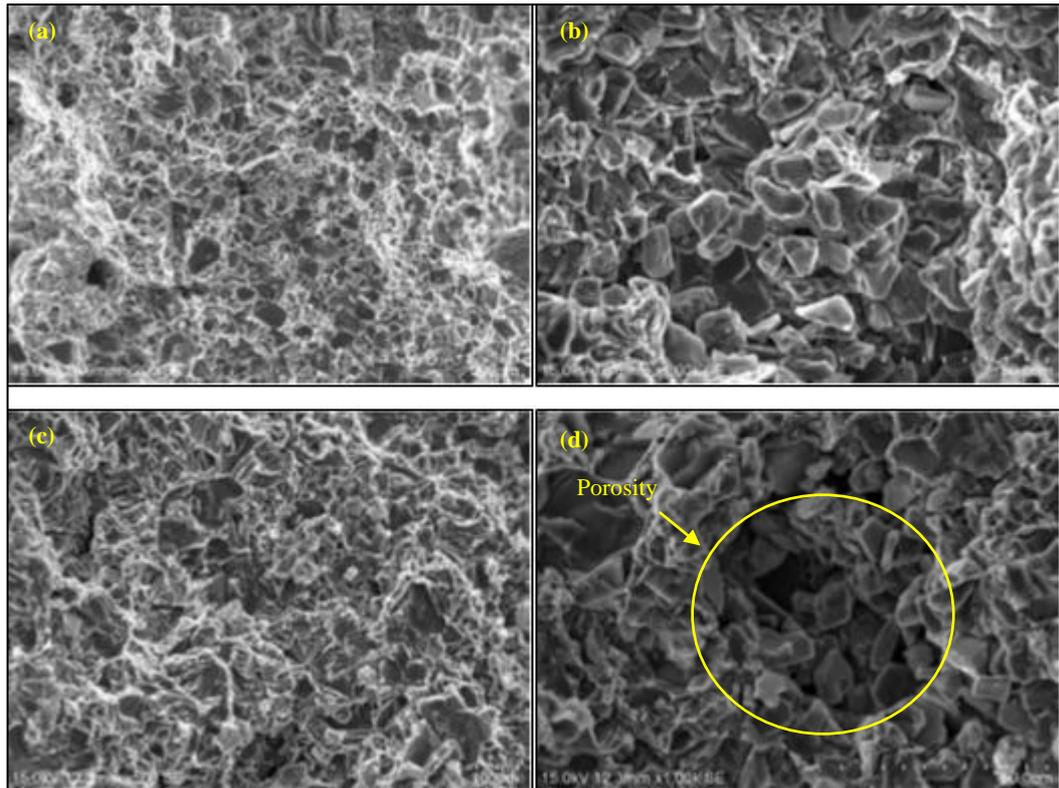
**Figure 5:** SEM micrographs of fractured in situ and hybrid MMCs with SiC content (a) 0 wt.% (b) 5 wt.% (c) 10 wt.% (d) 15 wt.%
