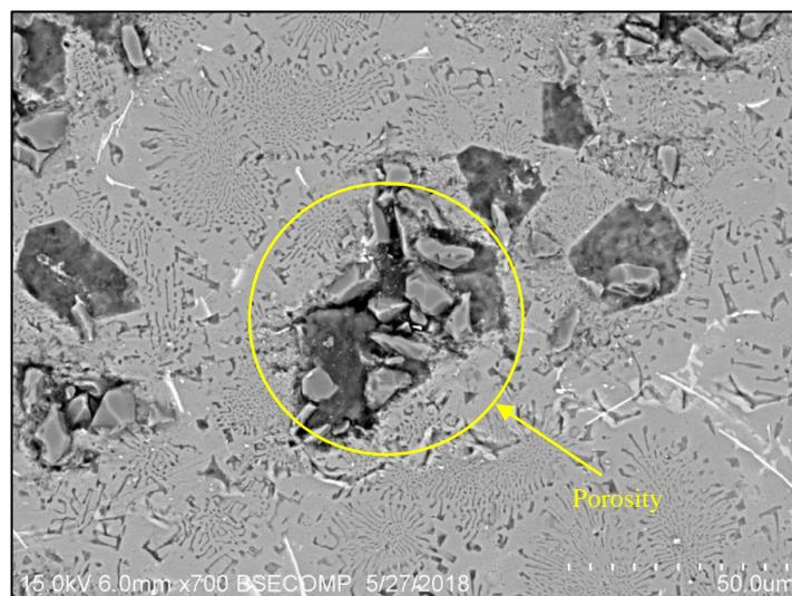
**Figure 3:** The presence of porosity in hybrid Al composite with 15 wt.% SiC
