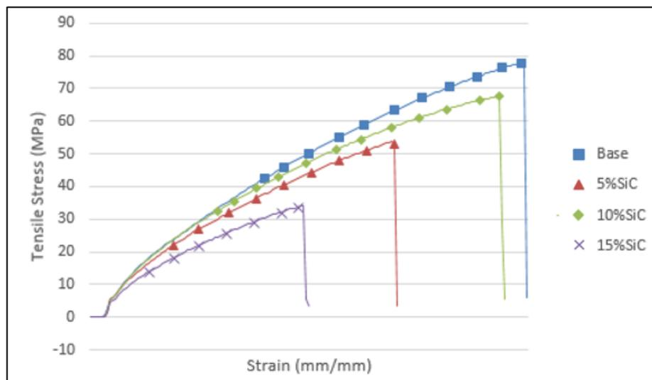
**Figure 4:** Stress-strain curve for all samples
