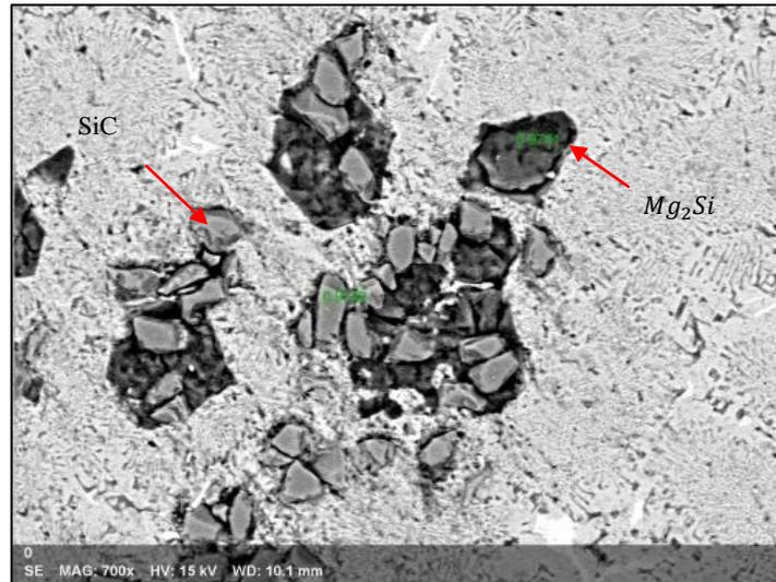
**Figure 2:** Validation of reinforcements' presence using Energy Dispersive X-Ray(EDX)
