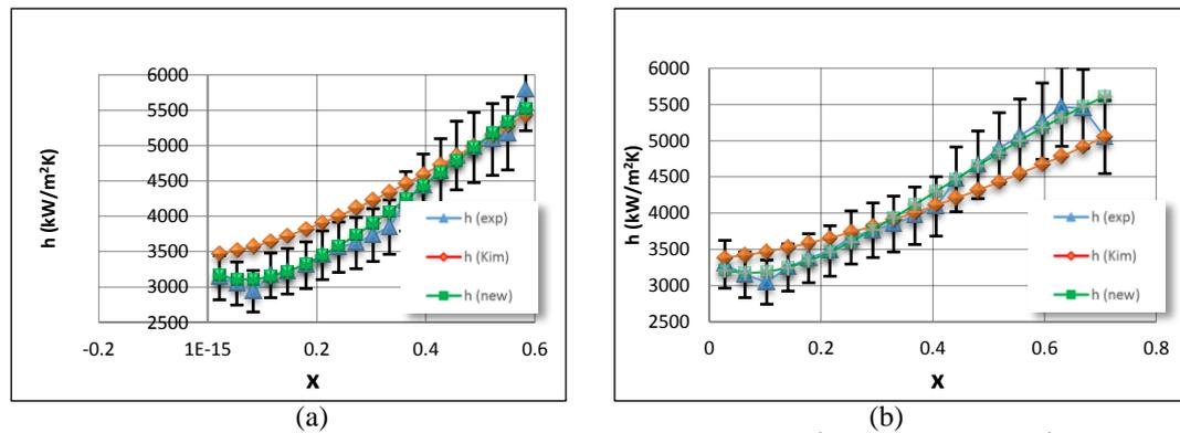
Figure 1: Graph  $h$  vs  $x$  with different  $G$  (a)  $G = 200 \text{ kg/m}^2\text{s}$  (b)  $G = 150 \text{ kg/m}^2\text{s}$
