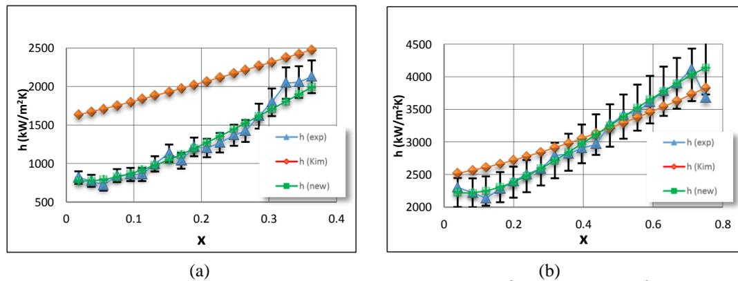
Figure 2: Graph  $h$  vs  $x$  with different  $q$  (a)  $q = 5 \text{ kW/m}^2$  (b)  $q = 10 \text{ kW/m}^2$
