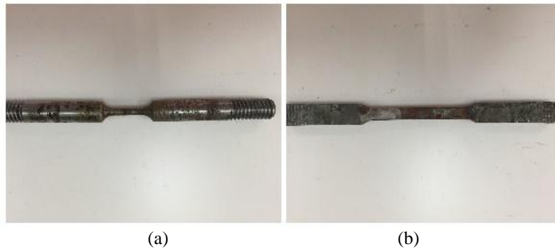
Figure 6: Test specimens after the SCC test for (a) round specimen and (b) plate specimen
