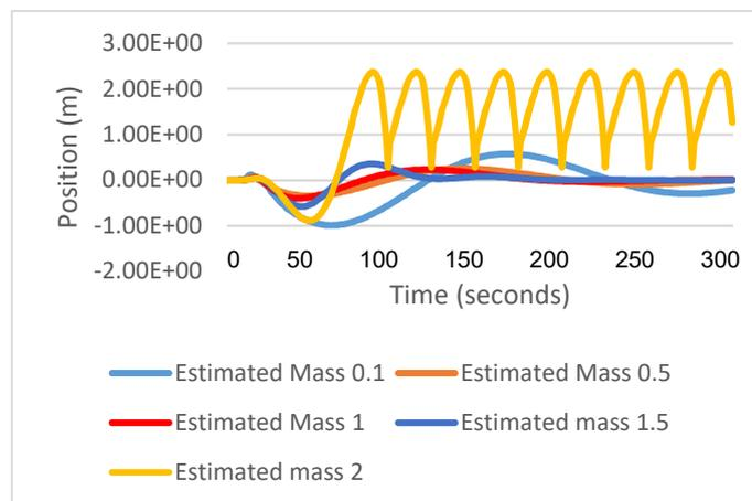
**Figure 8:** Estimated mass tuning in the AFC loop
