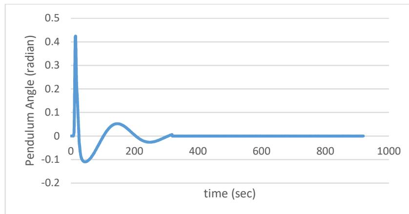
**Figure 5:** PID controller pendulum angle response
