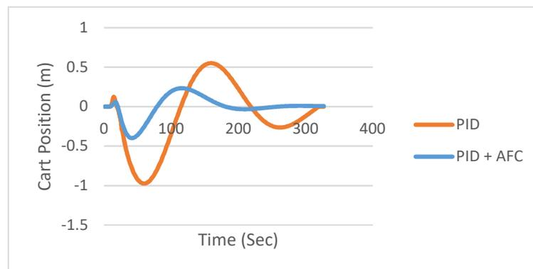
**Figure 11:** Comparison of cart position response between the two controllers
