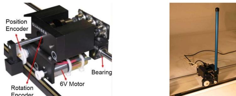
**Figure 13:** The actuator/sensor module (left) and the complete assembly (right) of the inverted pendulum rig
