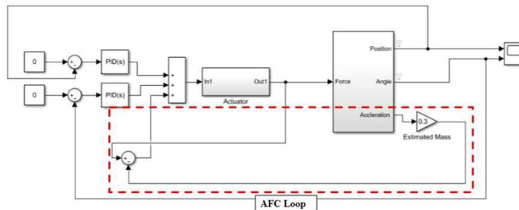
**Figure 7:** AFC loop as the inner loop of the overall control scheme
