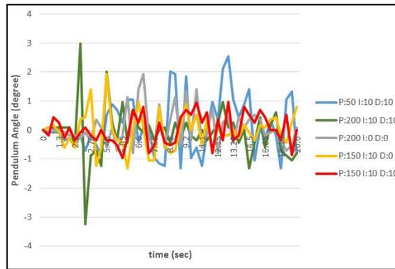
**Figure 15:** PID tuning for the pendulum angle
