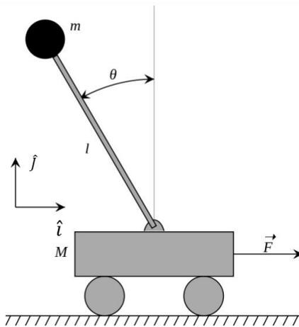
**Figure 1:** A representation of the inverted pendulum
