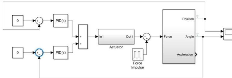
**Figure 4:** PID control loop for inverted pendulum
