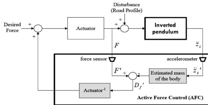
Figure 3: AFC loop for the inverted pendulum model
