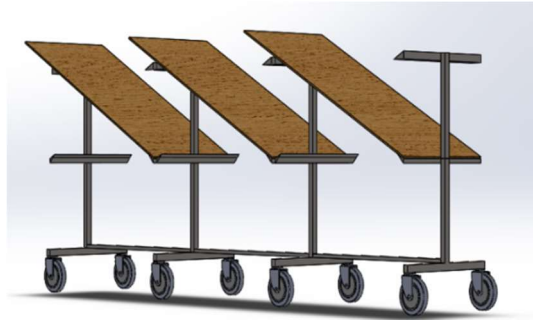
Figure 6: New platform design
