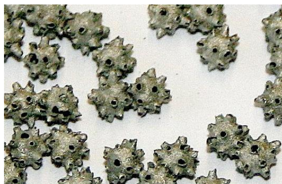
Figure 1 Photograph of the perforated hollow sphere structures production. (Photo from the courtesy of Glatt GmbH, Dresden, Germany)
