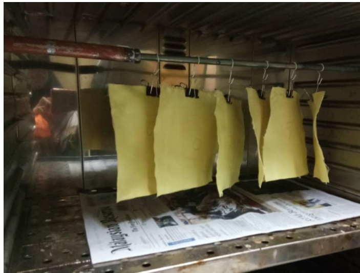
Figure 2: Evaporation of ethanol form impregnated fabrics in the oven
