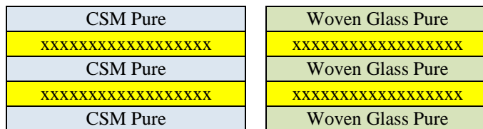
Figure 4: Stacking sequence for synthetic fibres intercalation with random short carbon fibres (random angle of aligned fibres)
