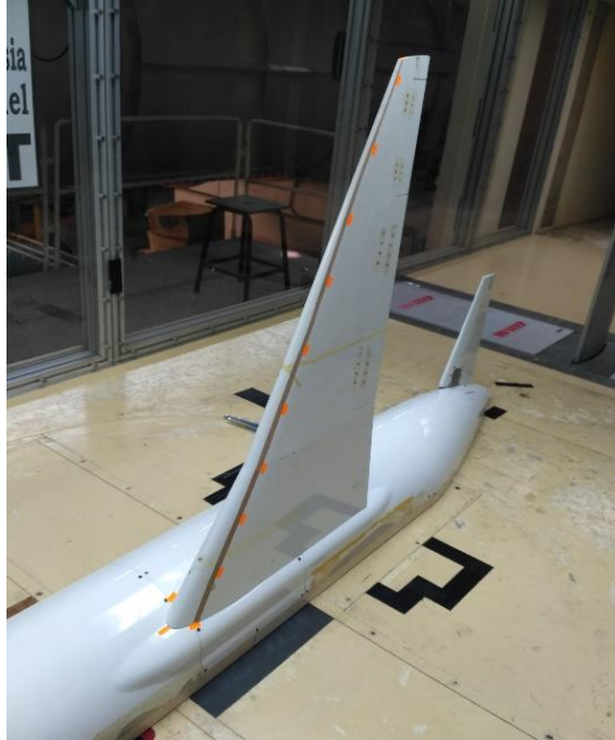
Figure 2: Ice roughness model location on leading-edge of the half model's wing
