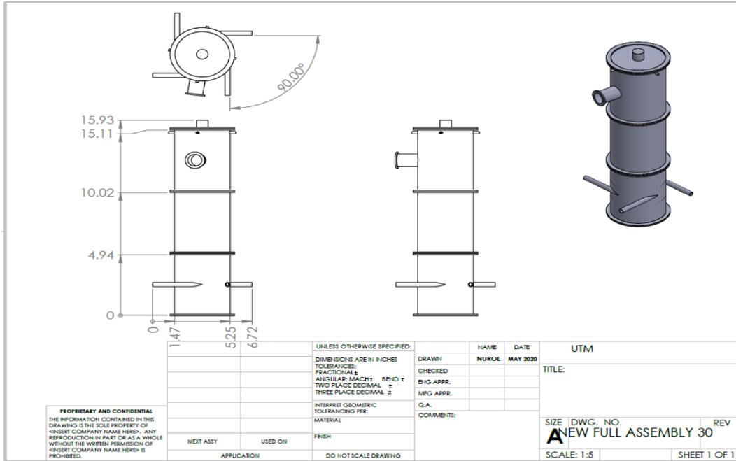
Figure 5 Assembly drawing for the reactor.
