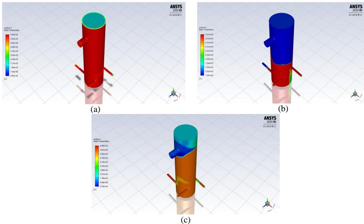
**Figure 9** Static temperature distribution at specific swirler angle. (a) 30°, (b) 40°, (c) 50° swirler.
