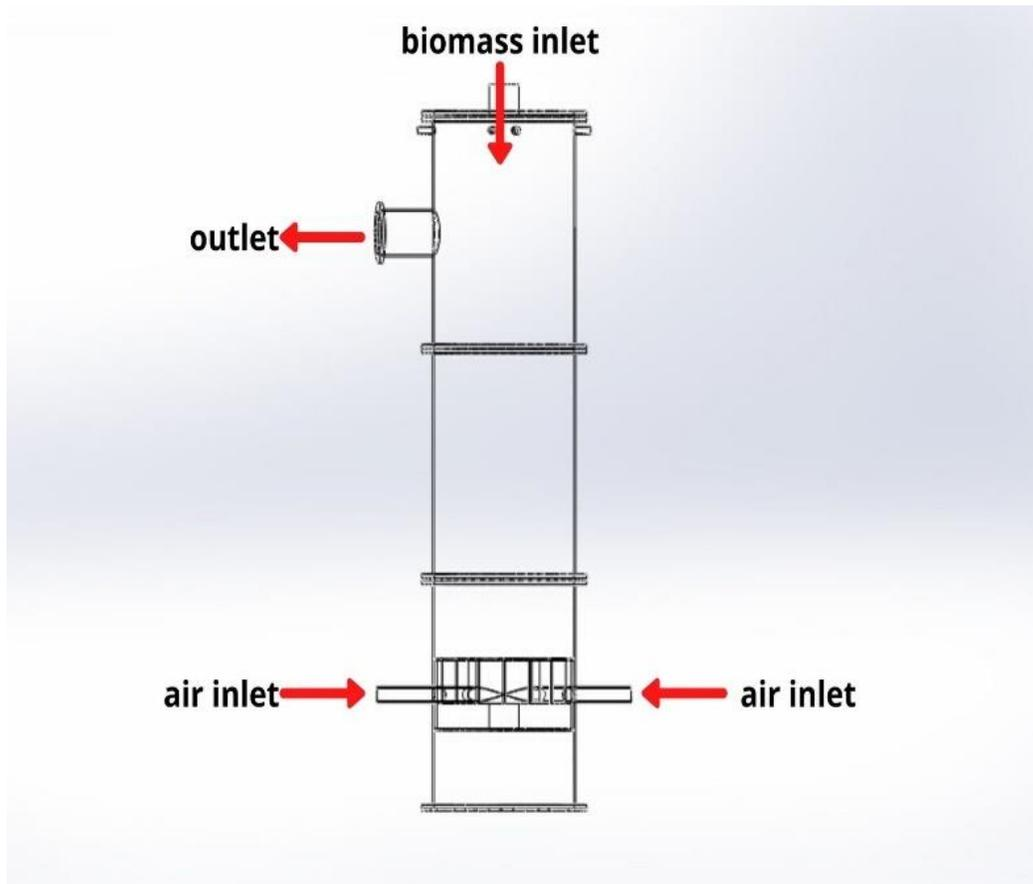
**Figure 4 Cross-section of chamber unit reactor.**
