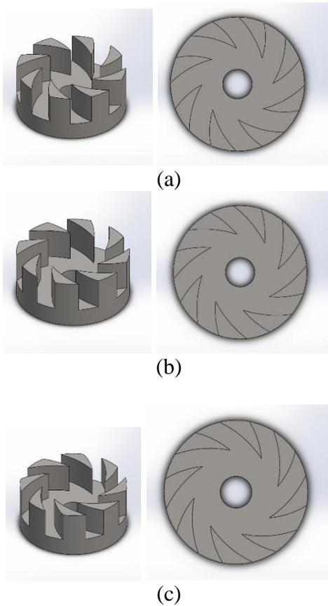
Figure 6 Swirler plate with angle (a) 30°, (b) 40°, and (c) 50°
