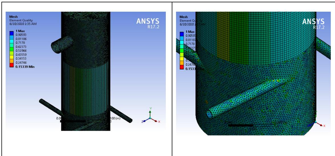
Figure 7 Meshing of Chamber unit
