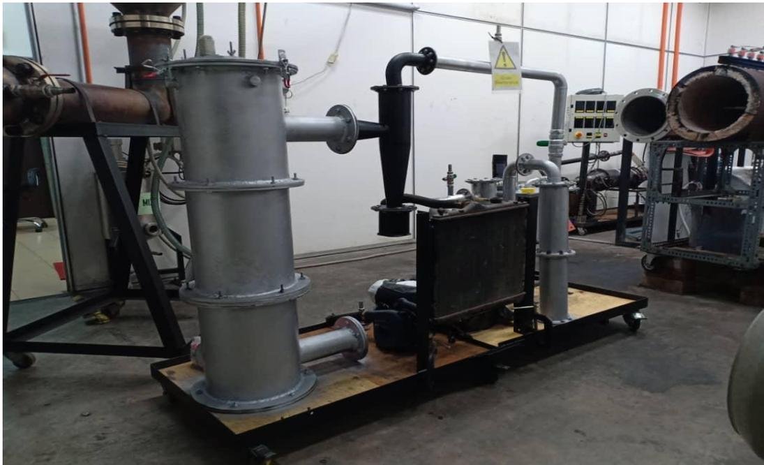
Figure 3 Fixed bed gasifier.
