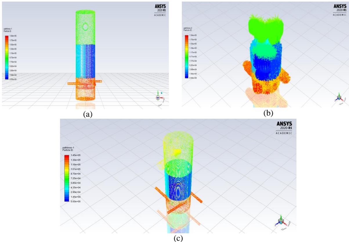
**Figure 8** Solid particle path line at specific swirler angle. (a) 30°, (b) 40°, (c) 50° swirler.
