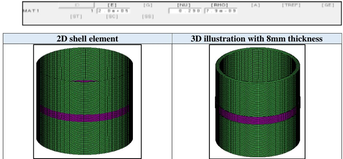
Figure 8: FEM for no crack
