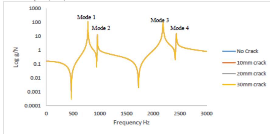
**Figure 10:** Comparison of the natural frequencies *Log vs Frequency* using FEA
