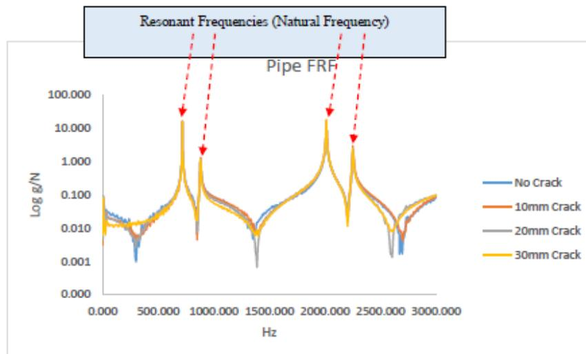
**Figure 12:** Comparison of natural frequencies *Log vs Frequency* using EMA
