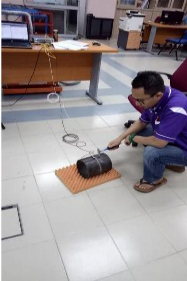
**Figure 7:** Excitation using an impact hammer (metal tip) on the CSP test specimen
