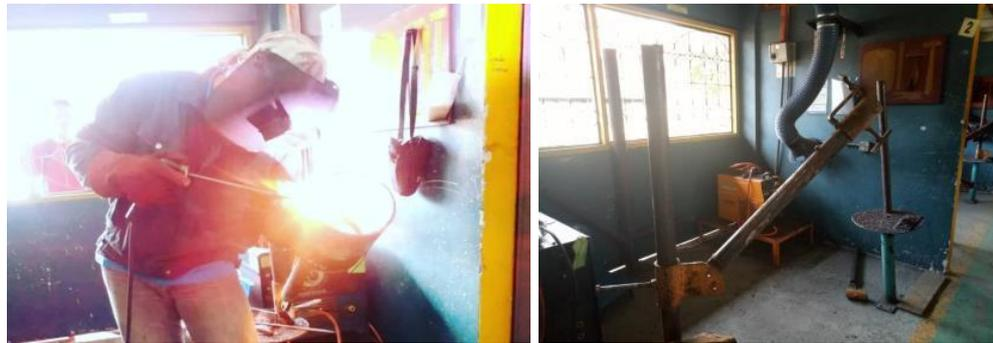
Figure 4: Jig and fixture for 6G pipe position
