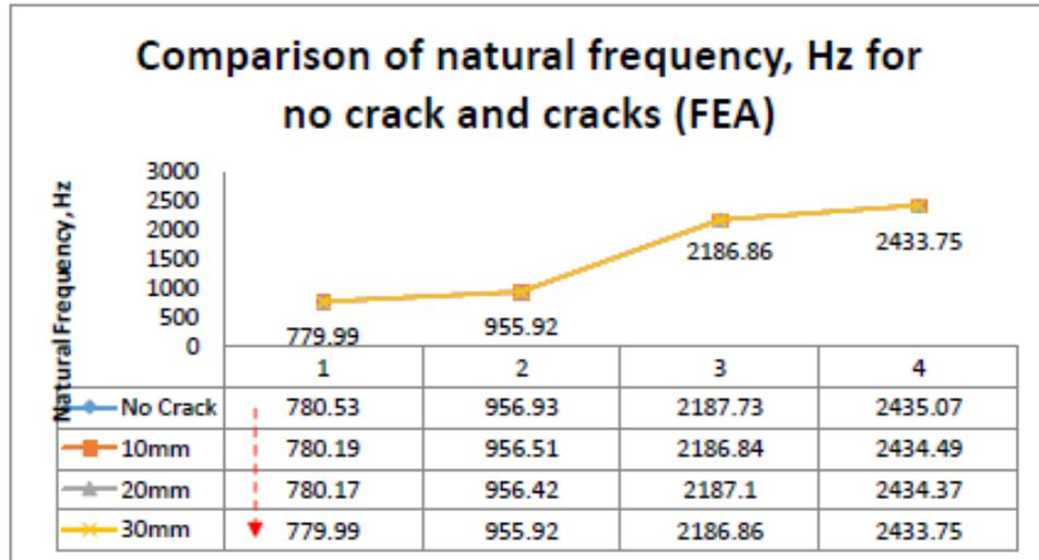
**Figure 14:** Comparison of natural frequencies for no crack and with cracks (FEA)
