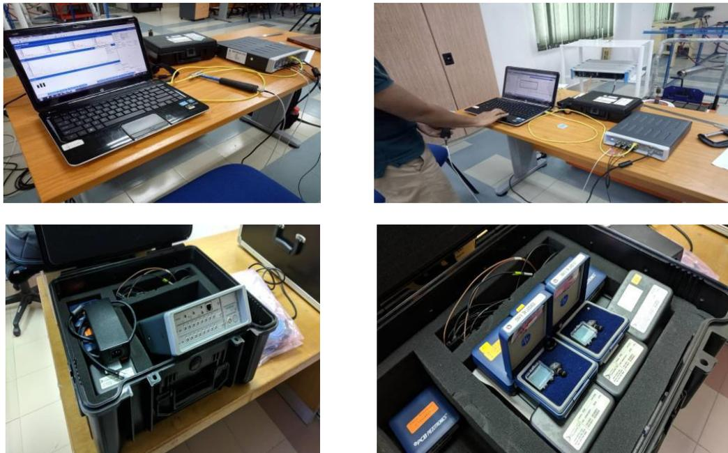
**Figure 6:** The *Bruel & Kjaer* Pulse Multi Channel Spectrum Analyser
