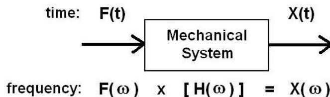
Figure 1: Block diagram of a FRF [4]
