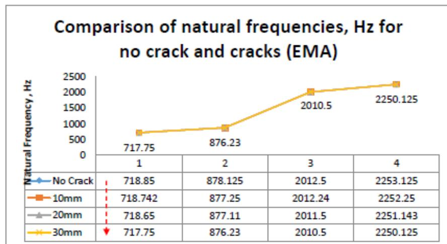
**Figure 13:** Comparison of natural frequencies for no crack and with cracks (EMA)
