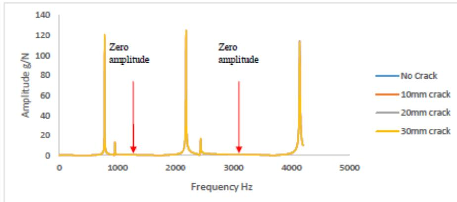
**Figure 11:** Comparison of the natural frequencies *Amplitude vs Frequency* using FEA
