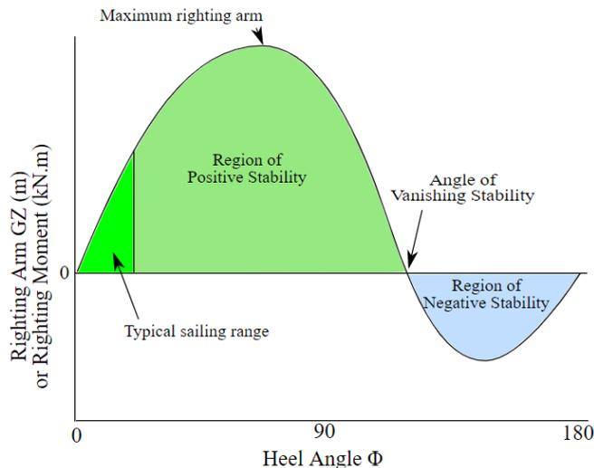
**Figure 5:** Righting Arm curve
