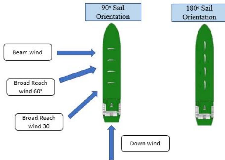
**Figure 12:** Apparent Wind Condition
