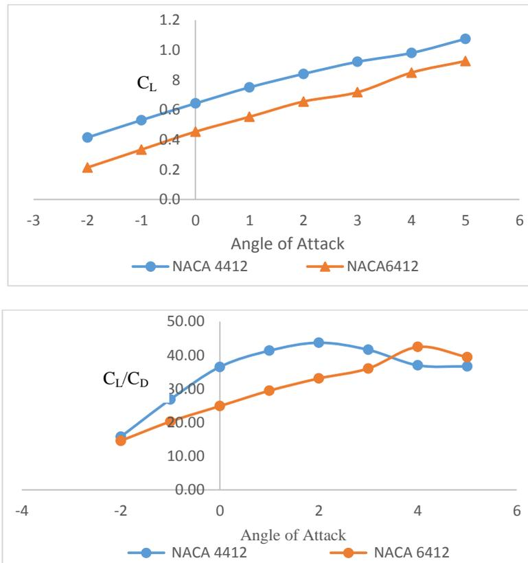
**Figure 9:** Coefficient of lift NACA 4412 and NACA 6412 vs angle of attack (top),  $C_L/C_D$  NACA 5412 and NACA 6412 vs angle of attack (bottom)
