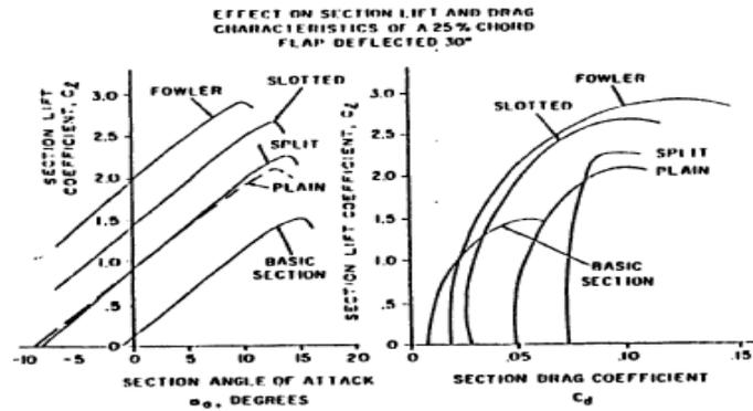
**Figure 4:** Effect of Flaps on Lift and Drag Coefficients [8]
