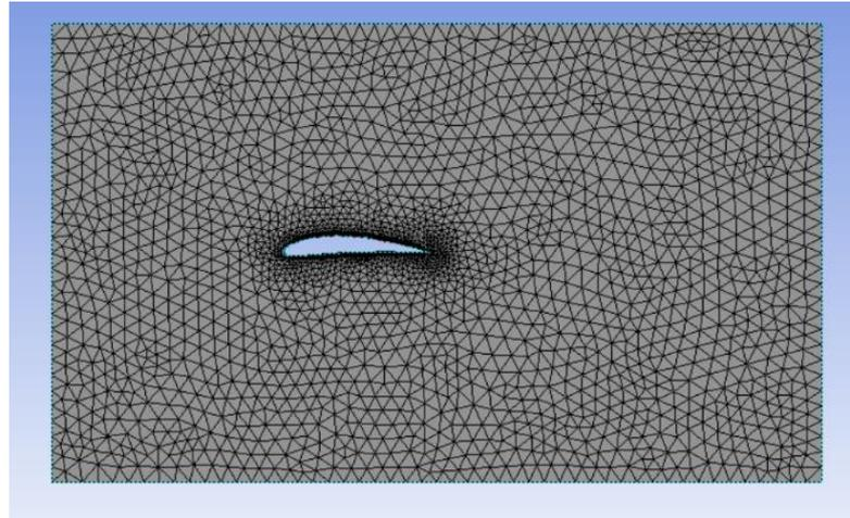
**Figure 7:** Meshing in ANSYS Fluent for the aerofoil
