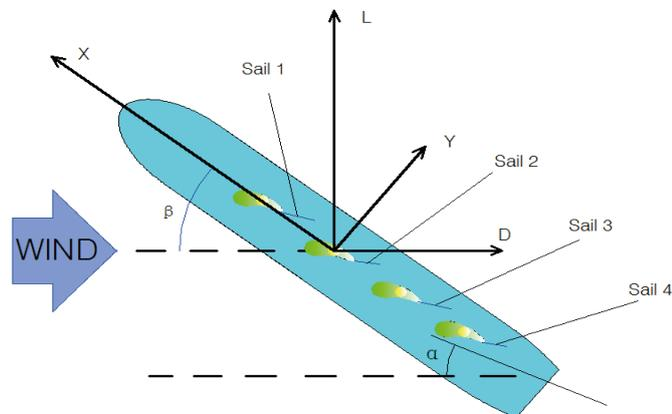
**Figure 1:** Coordinate system of the cascade sails for an imaginary ship [2]
