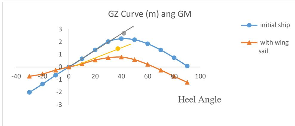
**Figure 19:** Comparison between GZ for initial ship and ship with sail
