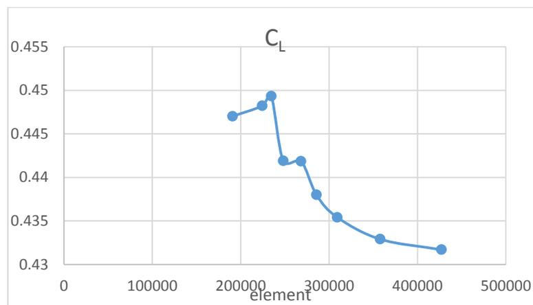
**Figure 8:** Grid Independence for NACA 4412 aerofoil
