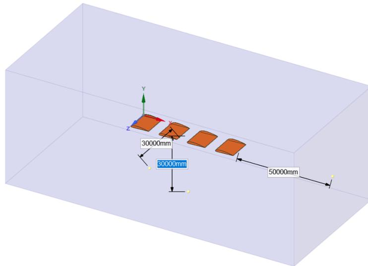
**Figure 11:** Domain Parameter of aerofoil
