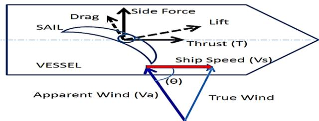
**Figure 3:** Forces acting on a wing sail [6]
