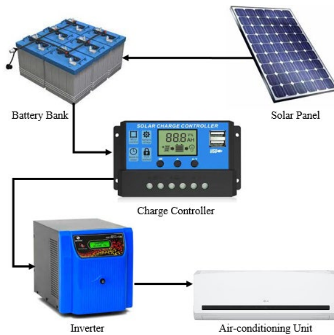
Figure 10: Schematic Diagram of Test Rig
