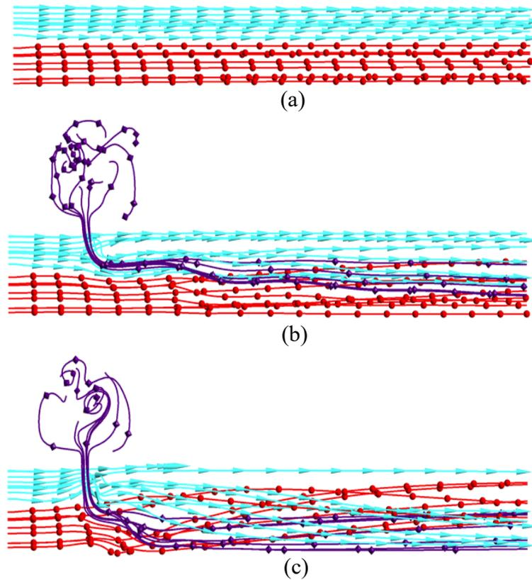
**Figure 4:** The streamlines pattern in the channel. (a) Case 1, (b) Case 2 and (c) Case 3
