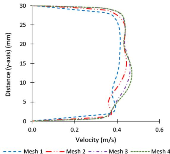
**Figure 3:** The velocity profile at 50mm away from inlet.
