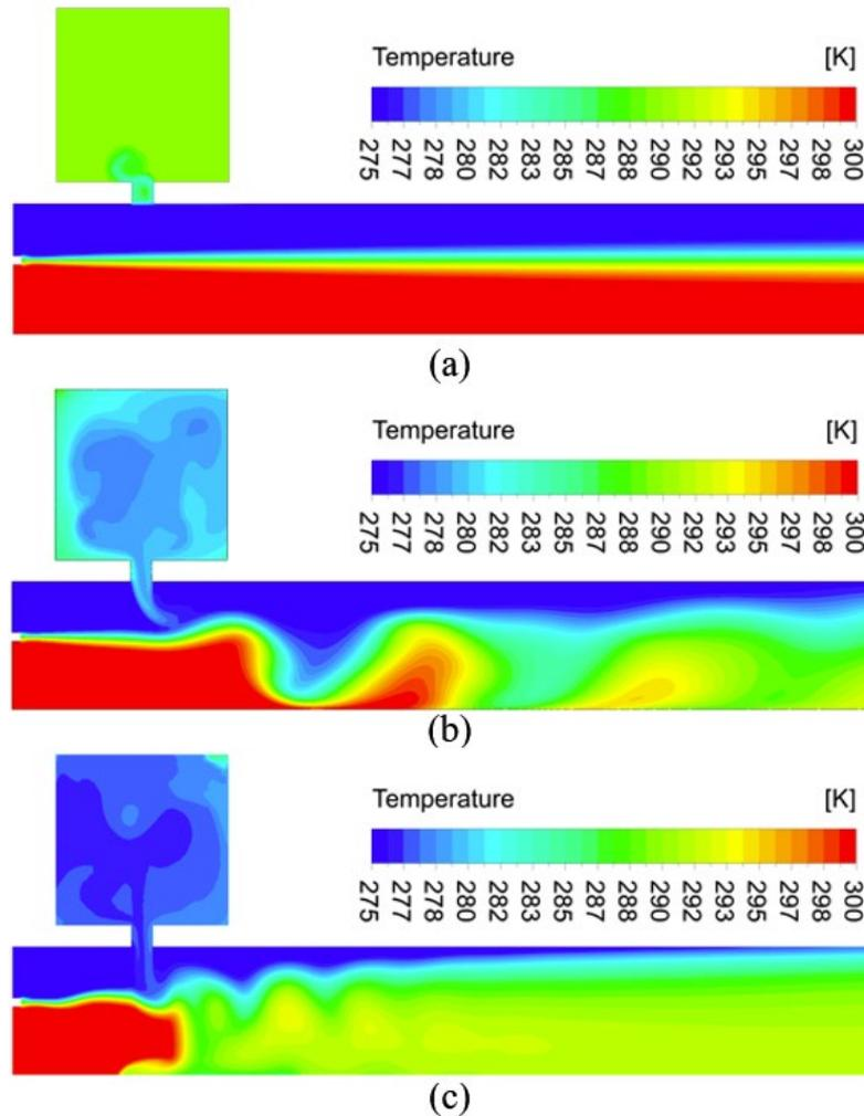
**Figure 6:** The contour of temperature distributions on the symmetrical plane. (a) Case 1, (b) Case 2 and (c) Case 3
