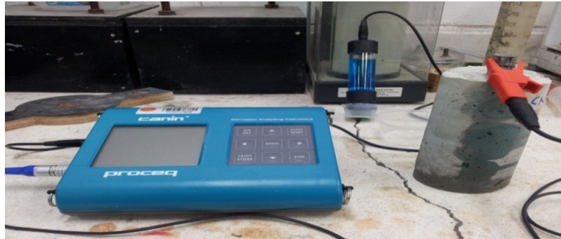
Figure 3 : Half-cell potential measurement set-up.
