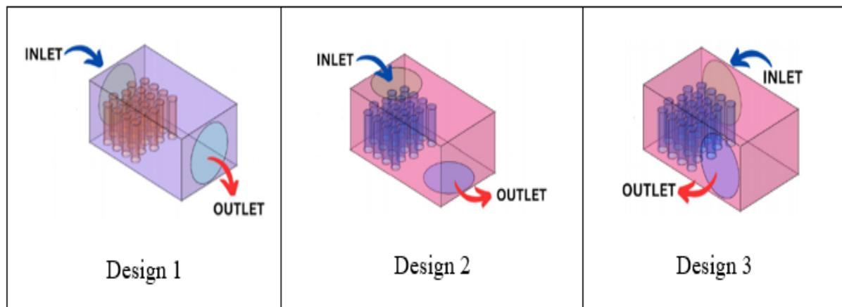
Figure 1: Ventilation design configuration
