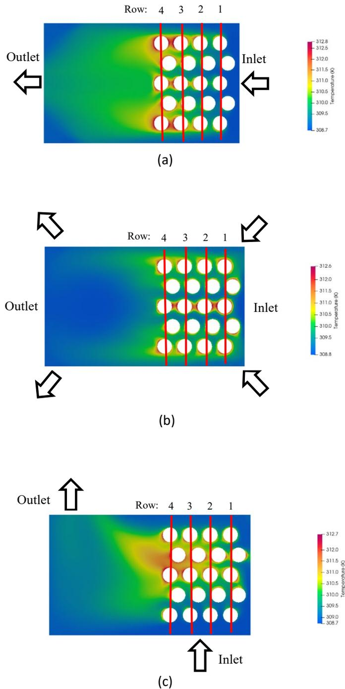
**Figure 2:** Temperature distribution for a) Design 1, b) Design 2, and c) Design 3 at inlet of 0.9 m/s
