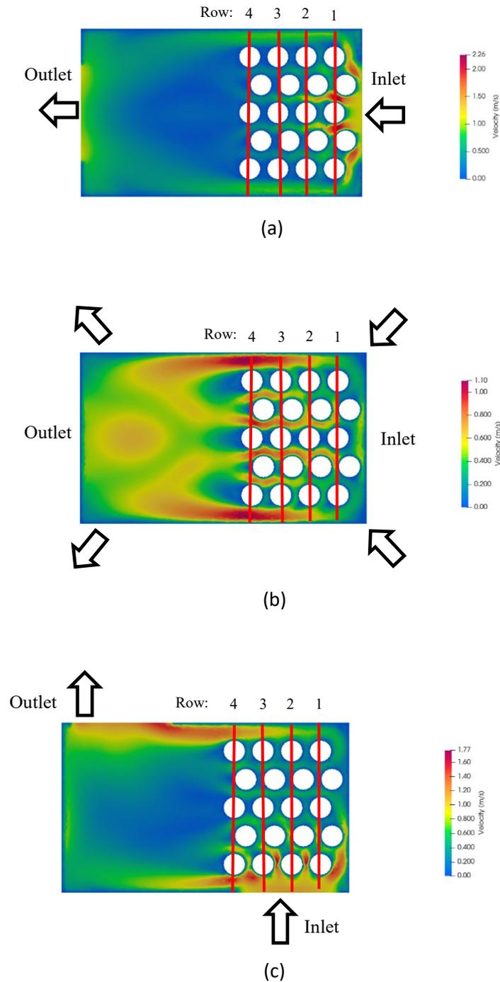
**Figure 3:** Velocity distribution for a) Design 1, b) Design 2, and c) Design 3 at inlet of 0.9 m/s
