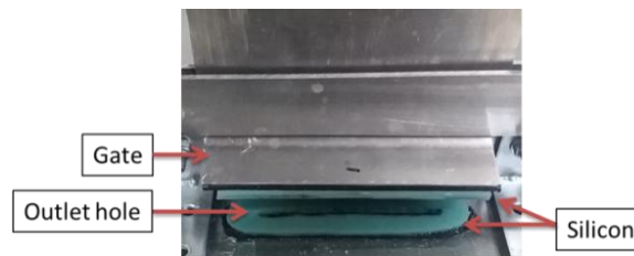
Figure 11: Paint gate sliding up view
