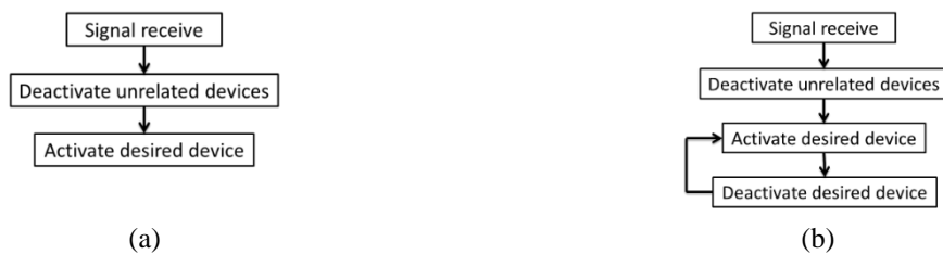
Figure 15: (a) General operation sequence in the void loop for 'if' function that receives the signal (b) General operation sequence in the void loop for 'while' function that receives the signal
