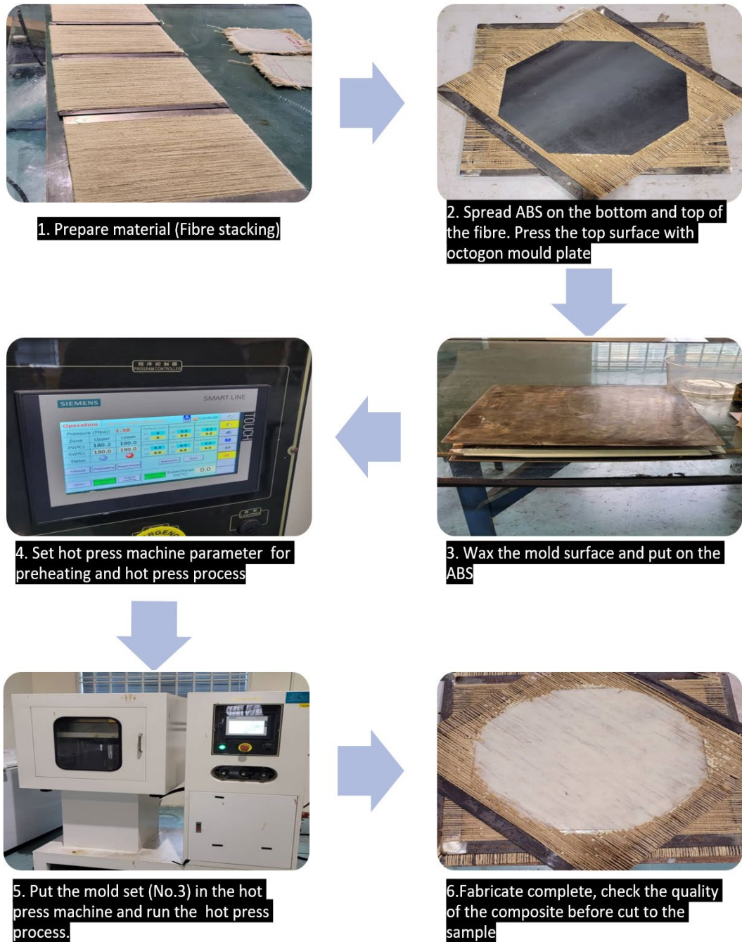
Figure 4: Hot compression moulding procedure.
