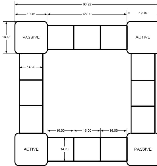
Figure 4. Semi-submersible main dimensions
