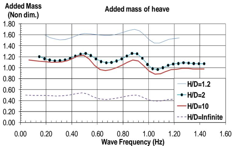
Figure 9. Added Mass of Heave for Different H/D ratio
