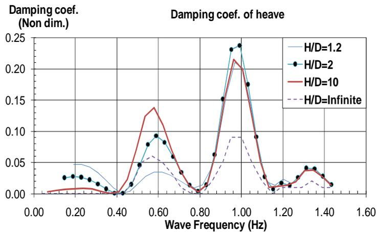
Figure 12. Damping Coef. of Heave for Different H/D ratio
