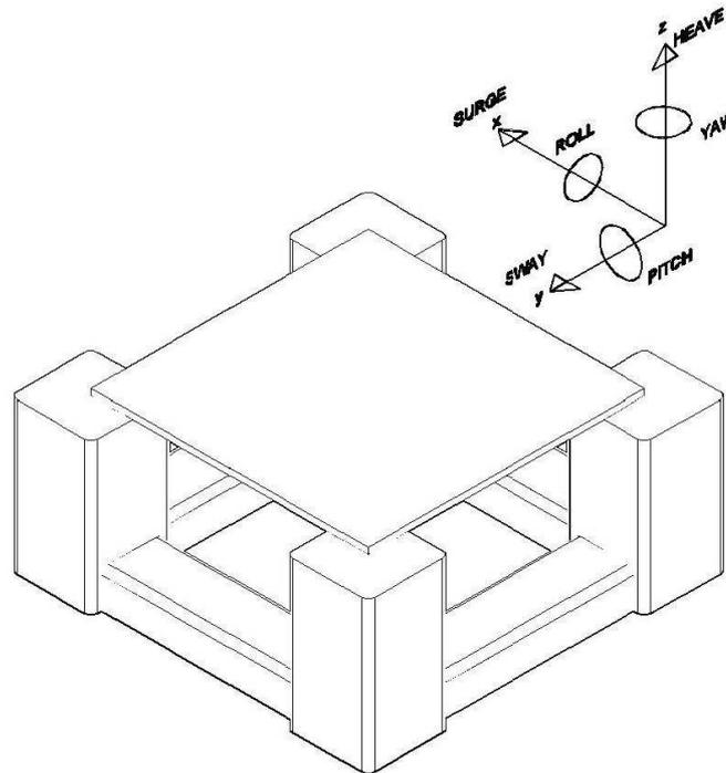
Figure 2: Semi-submersible motion definition
