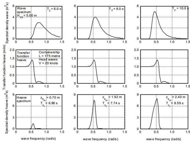
Figure 3. Effect of wave period on heave
