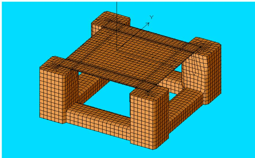
Figure 5. Modelling Semi-submersible in ANSYS AQWA
