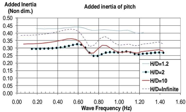
Figure 10. Added Inertia of Pitch for Different H/D ratio
