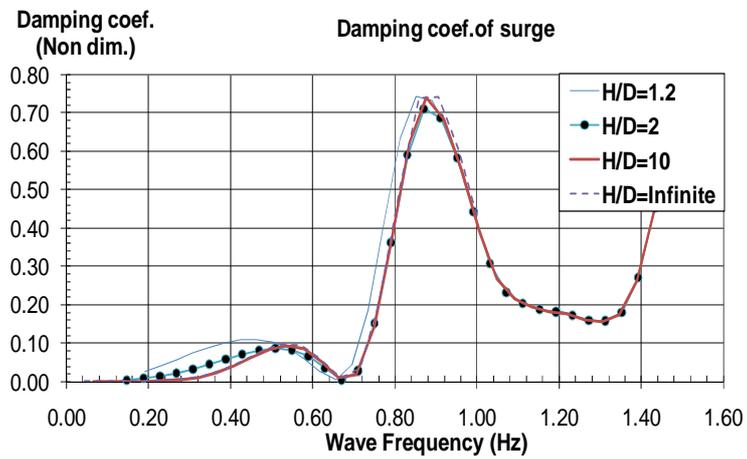
Figure 11. Damping Coef. of Surge for Different H/D ratio
