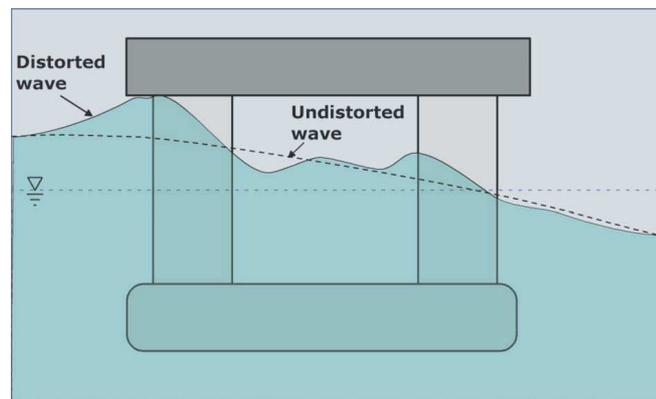
Figure 1. Schematic of wave run up problem
