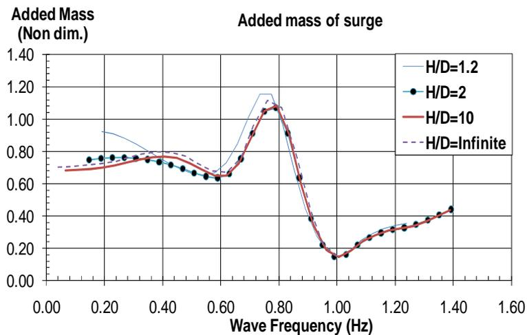
Figure 8. Added Mass of Surge for Different H/D ratio
