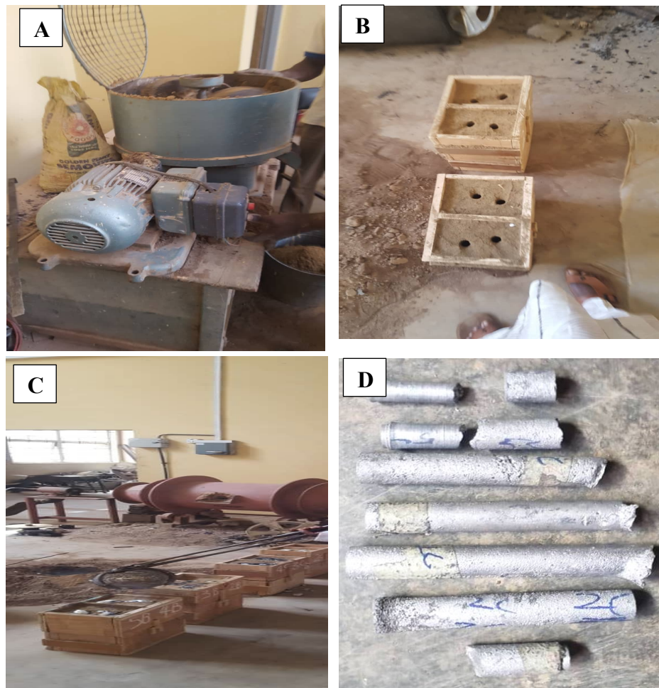
Figure 1: Casting Processes of the Aluminium Alloy
