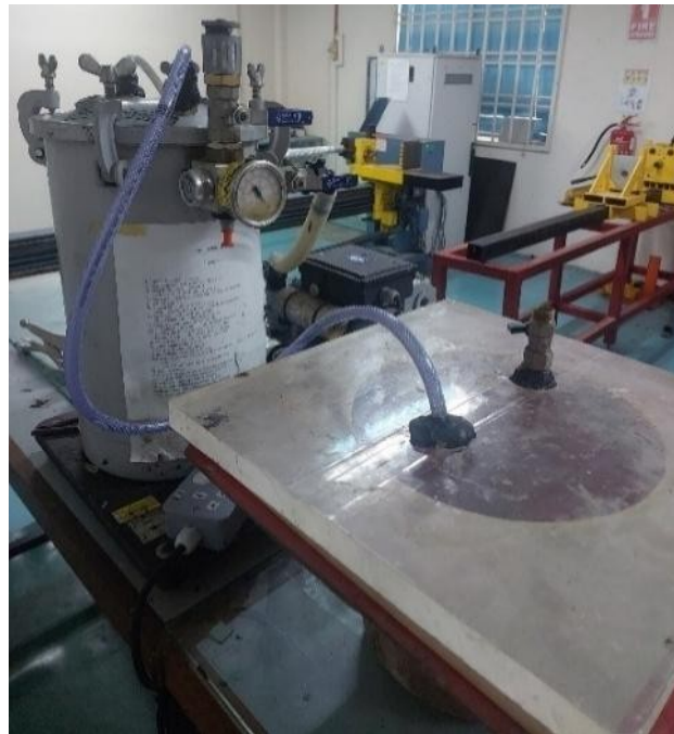
Figure 5: Process of removing air bubbles from the silicone mixture
