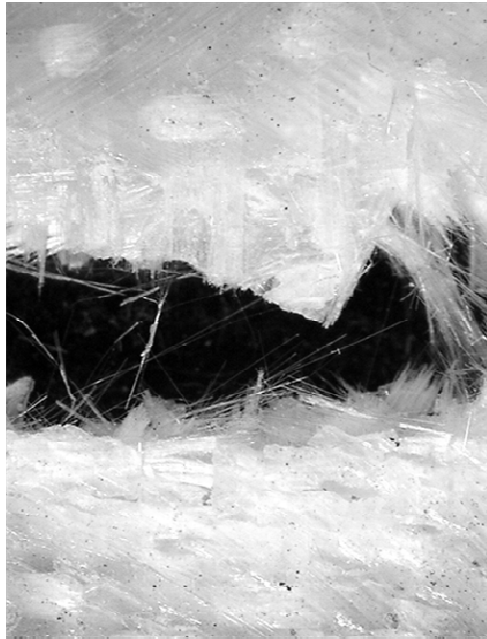
Figure 9 : Damaged [(0,60) 2 ]s Test Specimen
