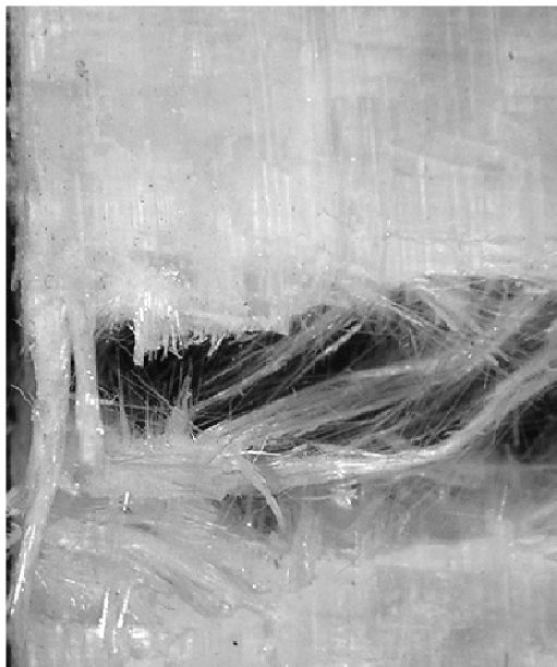
Figure 7: Damaged [(0,90) 2 ] s Test Specimen
