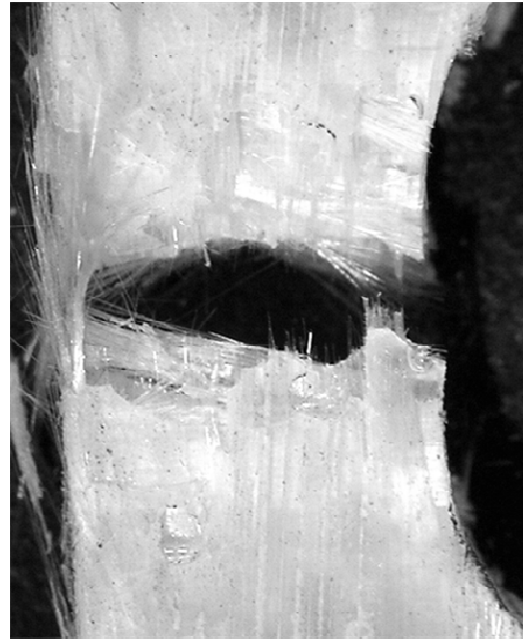
Figure 10 : Damaged [(0,90) 2 ]s Test Specimen with 10 mm diameter hole
