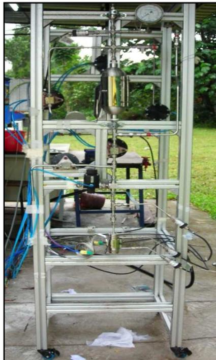
Figure 4 : Hydrogen peroxide rocket thruster facility.
