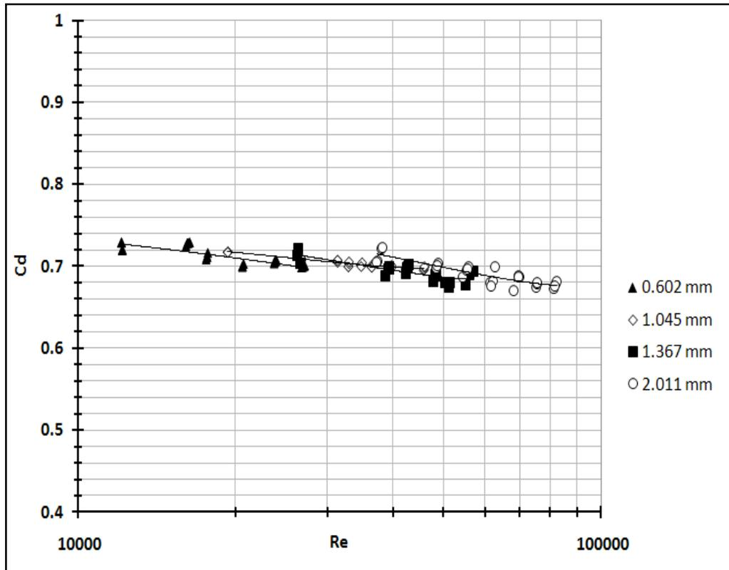
Figure 5 : Discharge coefficient for four different diameter injectors.
